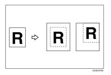
You can move the image to a corner or edge as well as center it. This function is useful when the copy paper is larger than the original.
